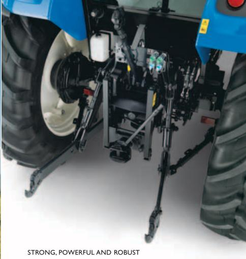
The rear linkage has been subjected to a stringent testing and rigorous quality control process to guarantee you top performance and reliability. The category two rear linkage has a maximum lift capacity of 3000kg for TD5.65 – TD5.75 tractors and a massive 3565kg for the remaining models, meaning you can work with the heaviest rear mounted implements with ease. For even more productive farming, specify the optional quick attach rear links for super-fast hitching from the comfort of the cab.
