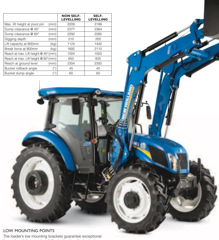
forward and downward visibility, both when the loader is mounted, or when it has been removed. Moreover, the low mounting points have lowered the tractor's overall centre of gravity, which improves stability when transporting full loads in the fully extended position.
